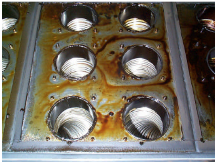
Following a 20-minute automatic self-cleaning cycle that does not interrupt production, the re-liquified flux is captured in collector trays that require replacement only once a year.
