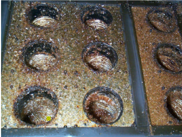
After 30 days of processing using 56.0 kg of solder paste, the condenser tubes in the flux collection system show significant flux accumulation.
