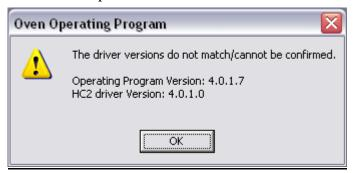
Make sure Oven and Oven Operating Program are not running while performing driver update. After finishing update restart power to controller by turning off and on the oven power.
